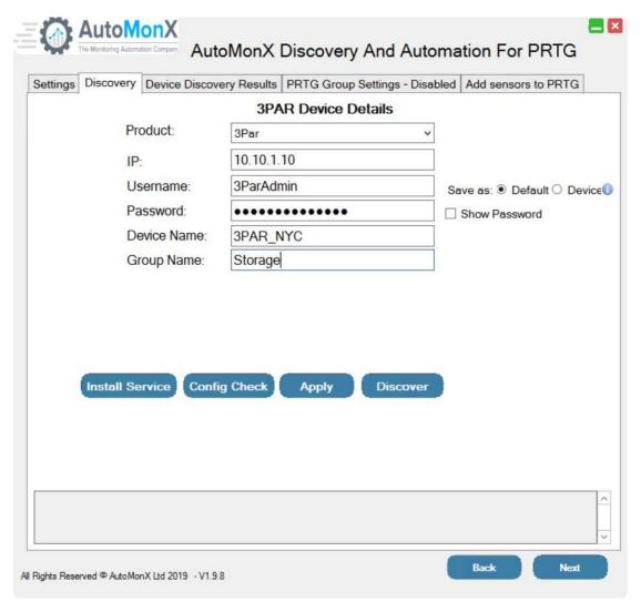
Save as Default – These credentials will be used for all 3PAR devices Save as Device - These credentials will be used for a specific device
